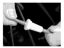
**NOTE:** The supply tube may be difficult to assembly to the filter body. Wiping the barb with water may facilitate assembly.
